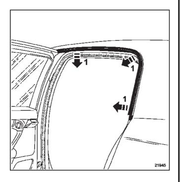
Using the tool (Car. 1363), unclip the trim (1).
